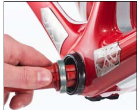
Figure 31. Pressing the bearing into the frame
